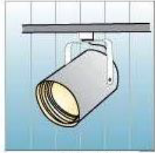
Track Lighting (Incandescent)
