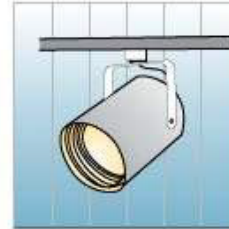
Track Lighting (Incandescent)
